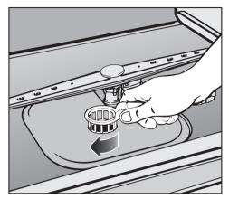
Turn the handle counterclockwise to release the filter combination.
